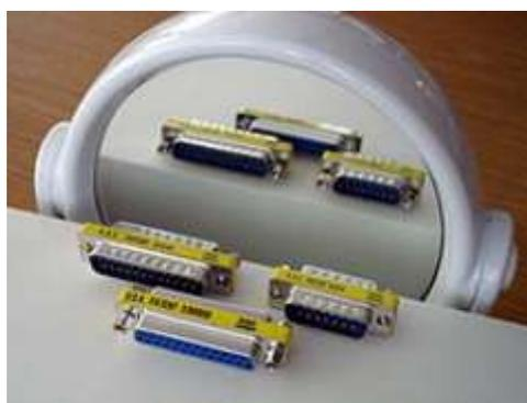
Figure 04: A Gender changer is a little piece of hardware that changes the 'sex of a computer cable'. Image of the hardware sourced at [http://en.wikipedia.org/wiki/Gender\\_changer](http://en.wikipedia.org/wiki/Gender_changer)
